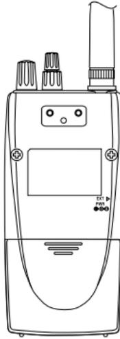
3. Press in on the ribbed area and slide the battery cover down and off.
