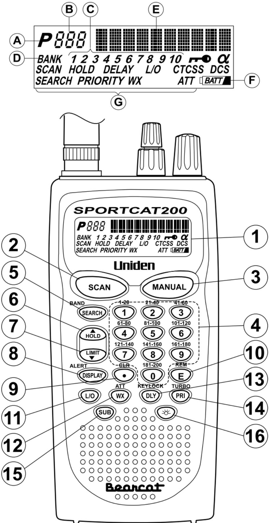
1. **LCD DISPLAY** — The liquid crystal display (LCD) shows the current channel and frequency. It also displays the mode, status, and bank indicators.
