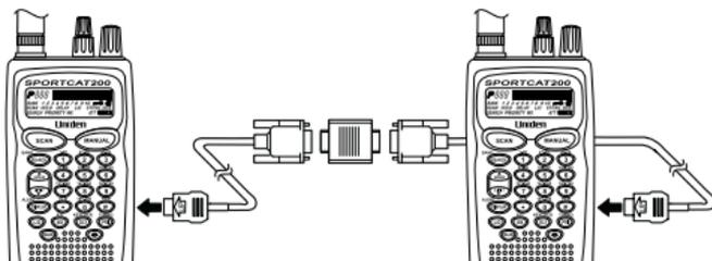
Plug the scanner end of the supplied remote interface cables into the remote ports on the right sides of each of the two scanners. When connecting the cable to your scanner, make sure the label side of the cable is facing forward.
