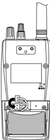
7. Replace the battery cover by putting the two tabs in the corresponding opening and sliding it upward until it locks in place.
