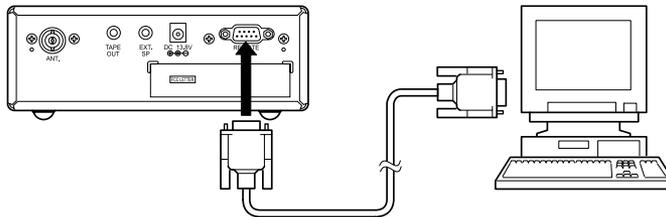
Plug the scanner end of the RS232C straight interface cable into the remote port on the rear of your scanner.
