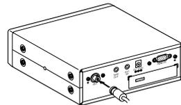
**Note:** If the antenna cable's connector does not fit in the **ANT.** connector, you might also need a Motorola-to-BNC antenna plug adapter (available at a local electronics store).
