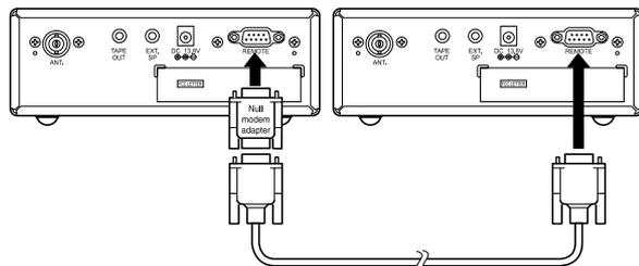
You can clone all of the programming of one BC780XLT into another, including frequencies, talkgroup IDs, alpha tags, delay settings, etc. After connecting the two scanners, turn the radios on. Prepare each scanner for clone mode as follows.
