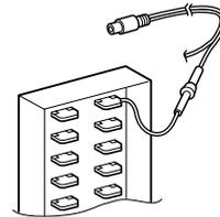
3. Insert the power cord's barrel plug into the **DC 13.8 V** jack on the back of the scanner.
